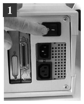
Locate the ON/OFF Switch and check that it is in the OFF position.
